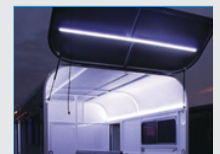
LED Internal Lighting
