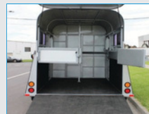
Rear breaching gates and barn door
